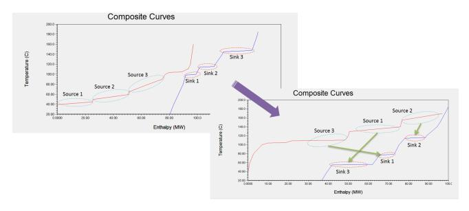
Example: Adjustment of process heat sources and sinks to maximize the heat recovery
